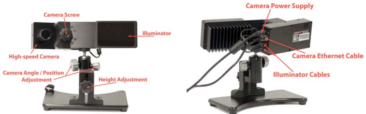
Figure 3-2: Parts of the EyeLink 1000 Plus Desktop Mount
